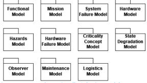
Figure 4: Proposed Functionally Cohesive model structure for RAMS.
